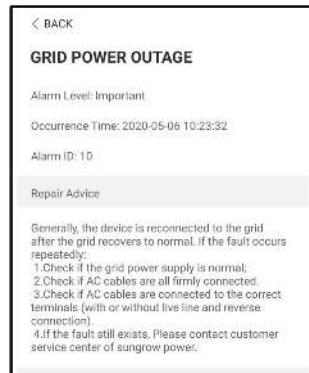
figure 7-9 Detailed Fault Alarm Information
