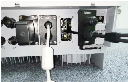
Step.3 connect the cable of new Meter & EMS cover to the RJ45 port of ET
