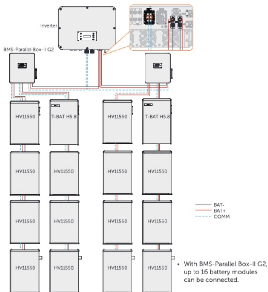
Figure 8-25 Battery connection with BMS-Parallel Box-II G2
